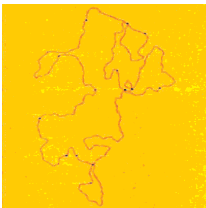
Fig. 3: AFM image of a mouse cosmid (35 kb) imaged in air. The dark spots on the DNA indicate individual EcoRI endonuclease molecules that bind to DNA molecules in a site specific manner. This illustrates the usefulness of AFM to study DNA-protein complexes and to map DNA sequences with site specific proteins under ambient conditions.
